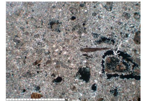
La20. Joining mortar. Early Spanish Colonial. Visible isotropic phases (likely silica gel). Left: PPL. Right: XP. Scale bar: 1 mm.
