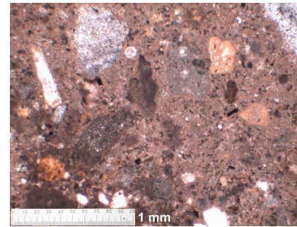
Ca36. Wall render. Late Classic. Micritic and crystalline calcareous aggregates. Lime lumps. Left: PPL. Right: XP. Scale bar: 1 mm.
