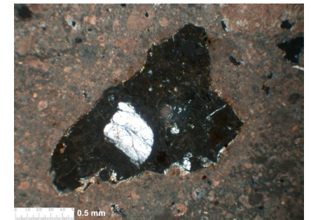
Pa27. Wall render. K'inich Kam Balam II. Impact glass with yellowish colour. Cracks, bubbles and sanidine grain can be seen. Hydraulic matrix. Left: PPL. Right: XPL. Scale bar: 0.5 mm. See appendix A.4 for composition of glass.
