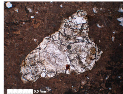
Pa27. Wall render. K'inich Kam Balam II. Impact glass with yellowish colour. Cracks, bubbles and sanidine grain can be seen. Hydraulic matrix. Left: PPL. Right: XPL. Scale bar: 0.5 mm. See appendix A.4 for composition of glass.
