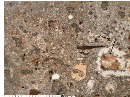
La20. Joining mortar. Early Spanish Colonial. Visible isotropic phases (likely silica gel). Left: PPL. Right: XP. Scale bar: 1 mm.
