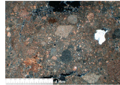
Pa49. Wall render. Otulum Phase. Hydraulic matrix, aggregates of micritic calcite and grain of quartz. Left: PPL. Right: XPL. Scale bar: 1 mm.
