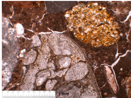
Pa28. Floor. K'inich Kam Balam II. Rounded reworked volcanic inclusion and rounded grain of biosparite. Clayey matrix. Left: PPL. Right: XP. Scale bar: 1 mm.
