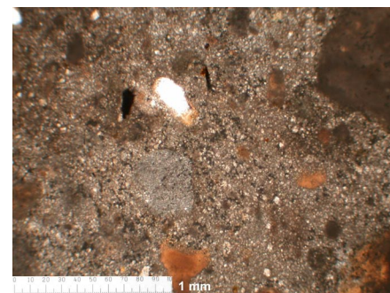
La40. Wall render. Early Spanish Colonial. Calcareous aggregates and orange partially isotropic phases (devitrified glass?). Left: PPL. Right: XP. Scale bar: 1 mm.
