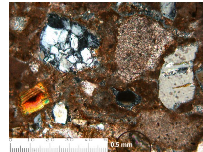
Pa88. Wall render. Otulum phase? Aggregates of crystalline calcite, polycrystalline quartz, feldspars and micas. Left: PPL. Right: XP. Scale bar: 0.5 mm.
