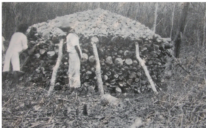
Fig. 3.9. Lime burning at Chan Kom. Picutre: Refield and Villa (1934).
