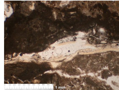
Ca29. Floor. Mineral from serpentine group. Left: PPL. Right: XP. Scale bar: 1 mm. See appendix A.4 for composition.
