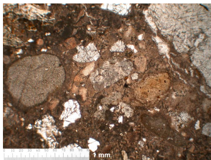
Pa12. Wall render. K'inich Kuk Bahlam II (Aka Kuk). Micritic and crystalline aggregates (some rounded) and isotropic phases. Left: PPL. Right: XP. Scale bar: 1 mm.
