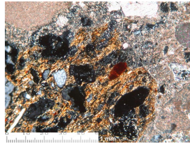
Pa 4. Joining mortar. Cascada Phase. Fragment of quartz-tempered ceramics (?) employed as aggregate. Left: PPL. Right: XPL. Scale bar: 0.5 mm.
