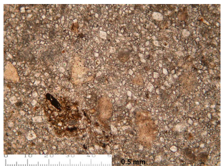
La21. Wall render. Early Spanish Colonial. Rhombohedral calcite, isotropic phases and clay pellets. Left: PPL. Right: XP. Scale bar: 0.5
