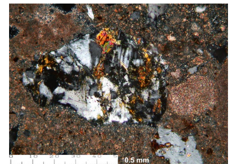
Pa53. Wall render. Balunté Phase. Rounded igneous rock with biotite mica, feldspars and opaques. Left: PPL. Right: XP. Scale bar: 0.5 mm.
