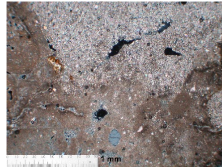
La 11. Floor. Terminal Classic/ Early Postclassic. Aggregate of crystalline calcite. XPL. Scale bar: 1mm.
