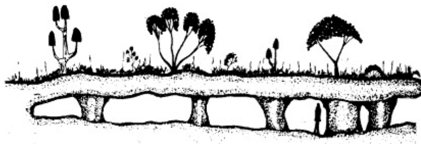
Fig. 3.2. Drawing of a sascab mine or sascabera . Image: Folan (1978). Columns are around 1 meter high.
