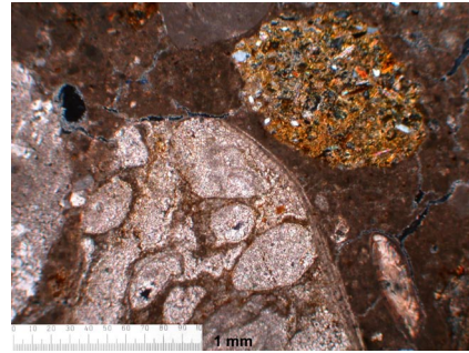
Pa28. Floor. K'inich Kam Balam II. Rounded reworked volcanic inclusion and rounded grain of biosparite. Clayey matrix. Left: PPL. Right: XP. Scale bar: 1 mm.
