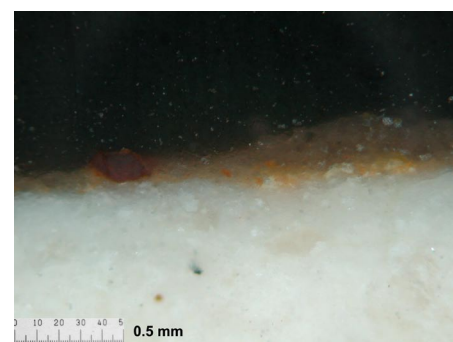
Ca8. Translucent pale yellow layer with orange-yellow particles. Scale bar: 0.5 mm
