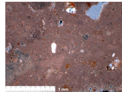
Pa78. Wall render. K'inich Janaab Pakal I. Aggregates of quartz and micritic calcite. A lime lump can be seen at the lower left corner. Left: PPL. Right: XP. Scale bar: 1 mm
