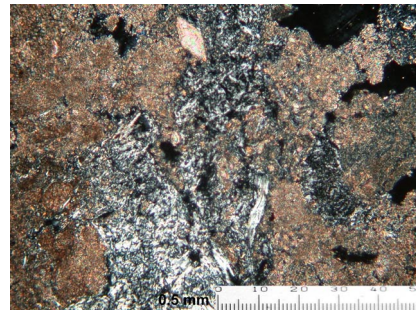
Ca9. Floor. Middle Preclassic. Masses of serpentine group mineral. Compacted sascab? Late Middle Preclassic. Left: PPL. Right: XP. Scale bar: 0.5 mm.
