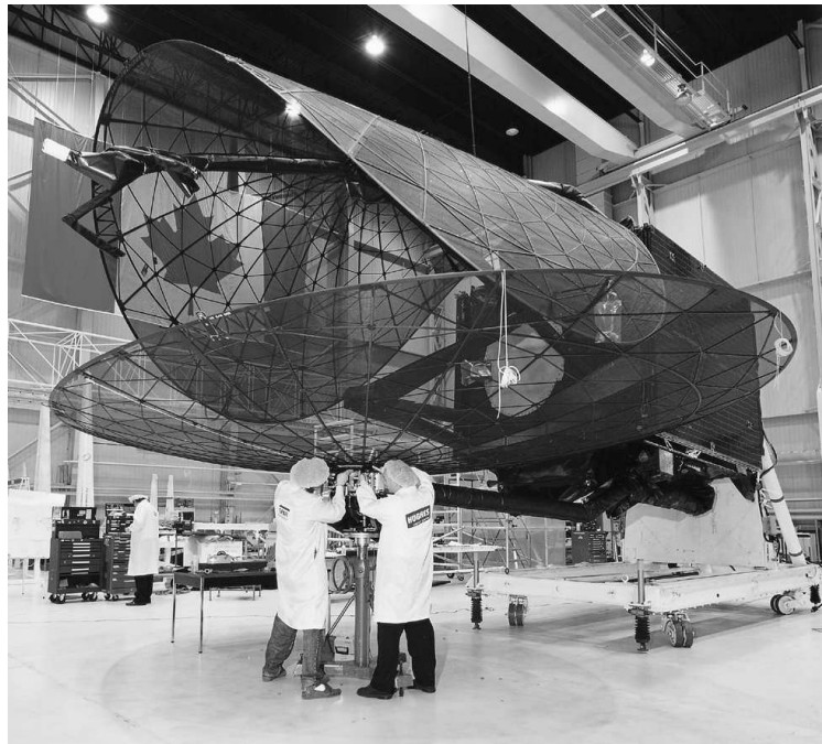
Figure 1. MSAT-2 spacecraft during ground testing with two Spring-Back Reflectors, one deployed and one folded. Courtesy of Canadian Space Agency.
