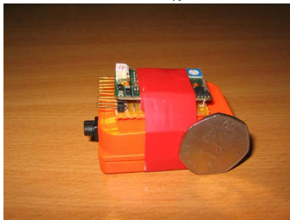
Figure 1 – A battery-powered MTx sensor connected to a connectBlue WiFi module via RS232
