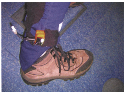
Figure 2 – An illustration of the position of the sensor (securely placed to a pocket of the right shank of the tracksuit)
