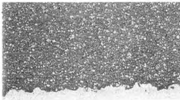
Figure 85 Tool steel base powder Coating on D2 Steel with sand blasting surface roughened
