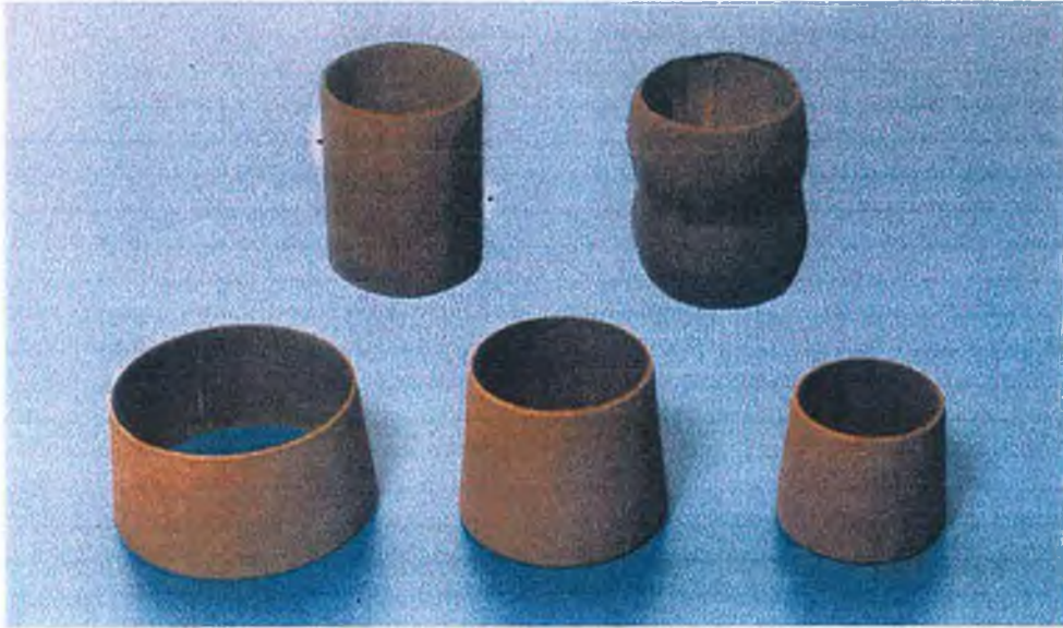
Figure 20 Pictures of cylindrical components manufactured with HVOF process
