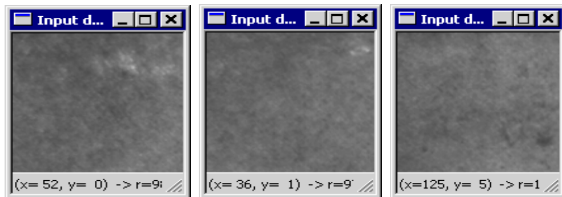
Figure 10. Image sections with acceptable finish but presenting a small but acceptable shade variation.
