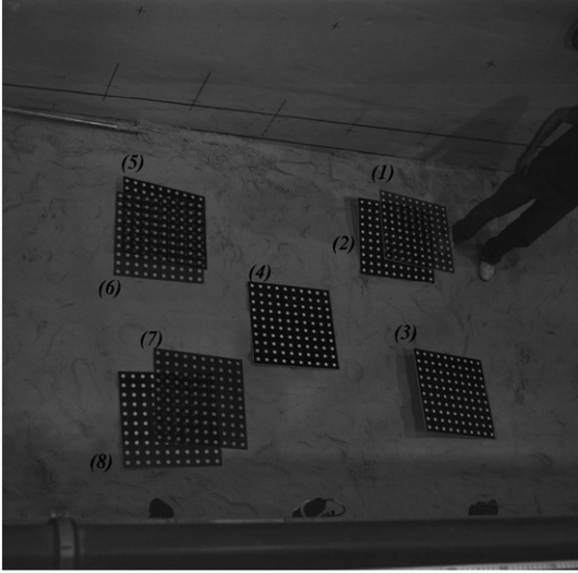
Fig. 7. The 8 different views superposed on one image of the model plane for the global calibration of the stereovision system.
