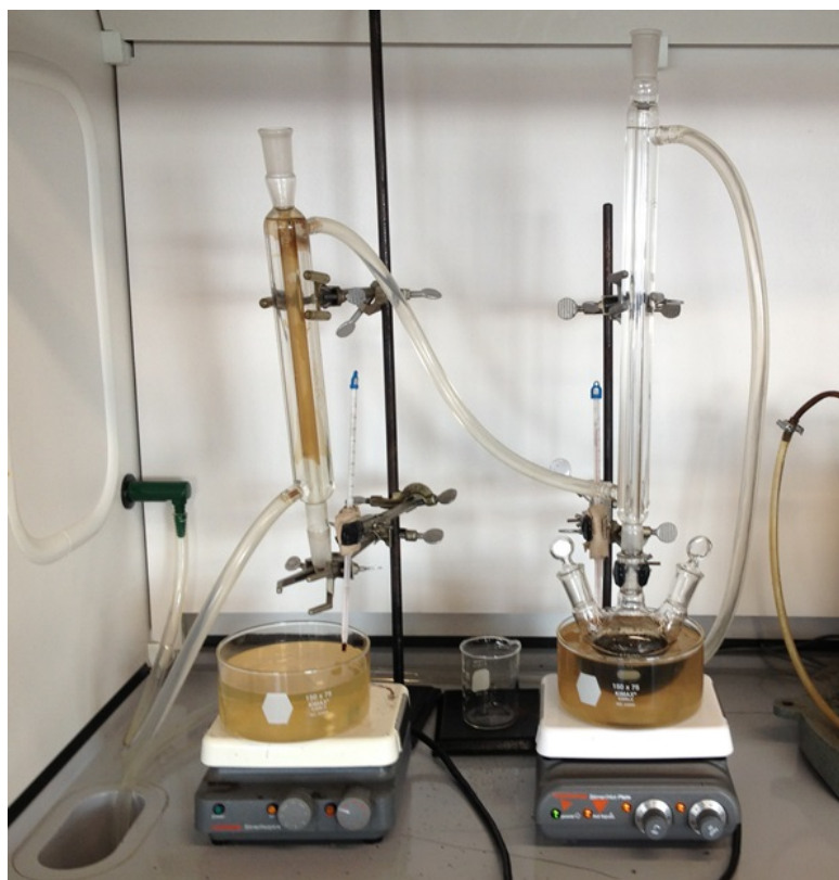
Figure 9: Photo of the solvent extraction apparatus used
