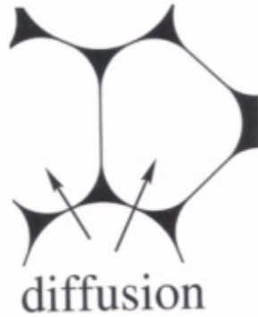
Figure 2.2. Diffusion of gas from bubble through the film. The plateau border acts as a barrier for diffusion [49].
