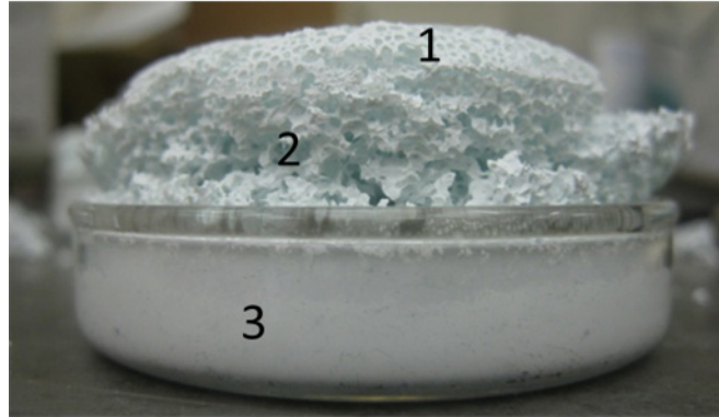
Figure 6.1. Image of pre-sintered foam to illustrate the 3 regions produced. 1) 'surface region', 2) 'foamed region' and 3) 'dense region' which is ceramic that did not foam during the emulsion process.
