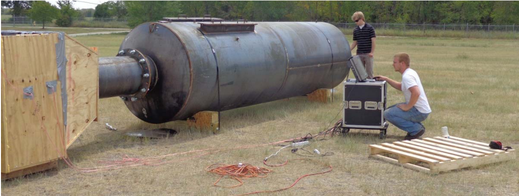
Figure 2.7: Corporate site measurement setup of mid-size muffler model
