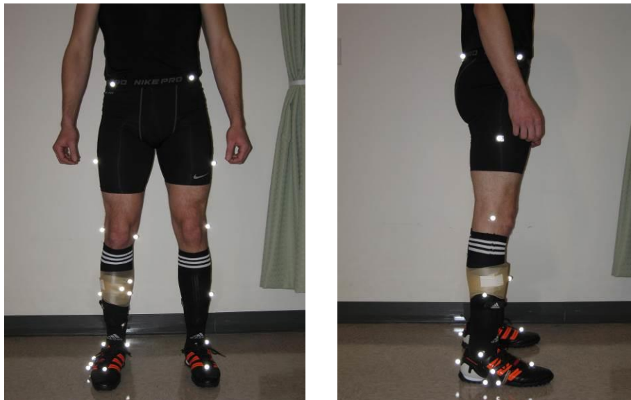
Figure 21. Modified Plug-in-Gait Marker Set. Additional to the lower extremity Plug-in Gait marker set were medial epicondyle, medial malleolus, tibial sensor triad, foot sensor triad of the dominant leg.
