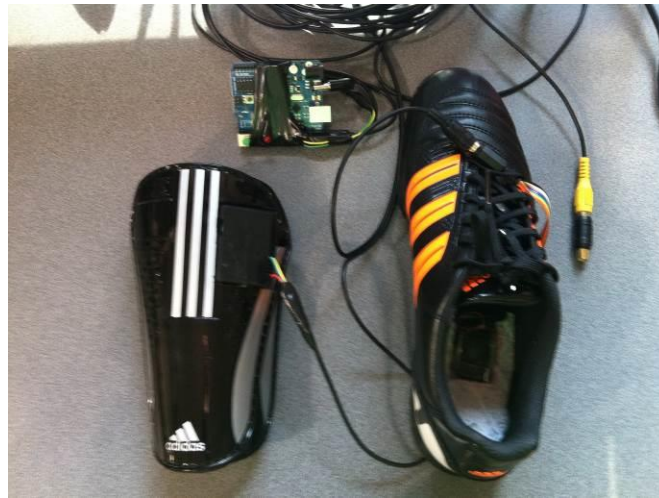
Figure 17. Instrumented equipment with synchronization trigger
