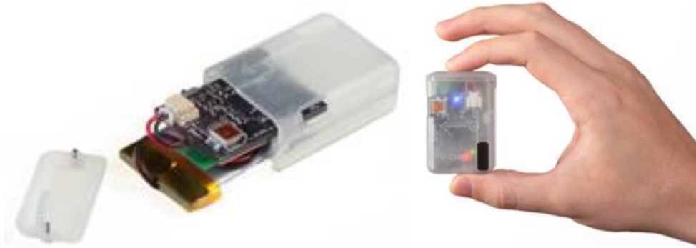
Figure 8. x-IMU with plastic housing and 1000 mAh lithium polymer battery.
