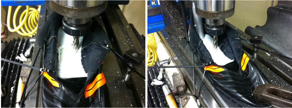
Figure 11. Milling of turf shoe insole to integrate the MARG
