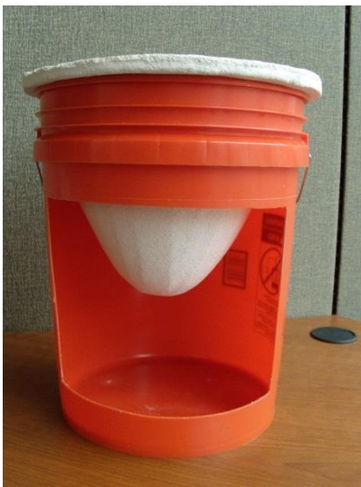
Figure 2: Ceramic filter element in a 5 gallon bucket.
