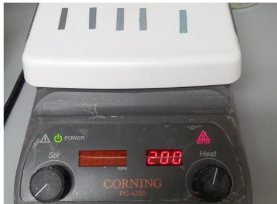
Figure 14: AgNP deposited wafer samples undergoing heat treatment
