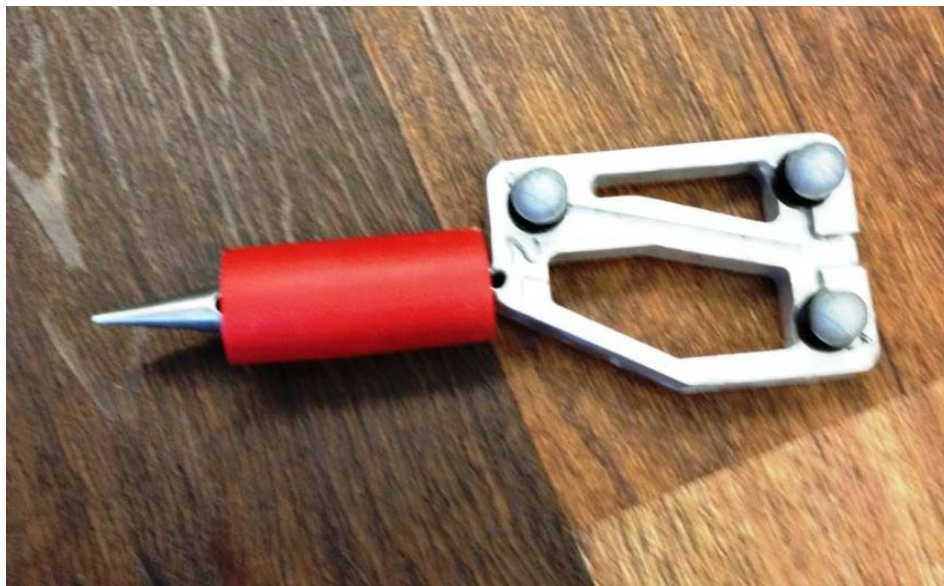
Figure 15: Digitizing Stylus with Vicon Markers
