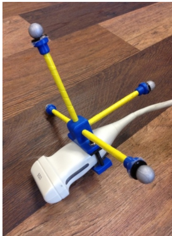
Figure 4: Ultrasound probe fitted with custom orthogonal attachment and Vicon markers
