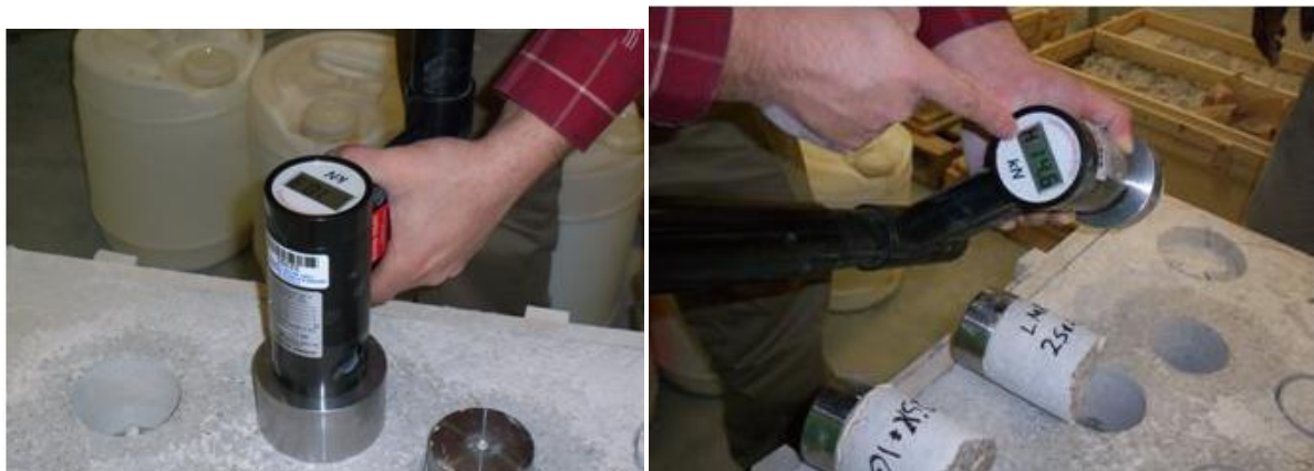
Figure 3.17. Direct tensile bond strength test.
