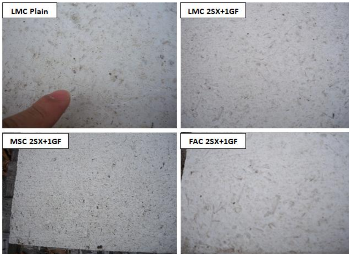
Figure 3.19. Close-up view of the surfaces of the segments around the edges after 2 years of sitting outside the lab in an open environment.
