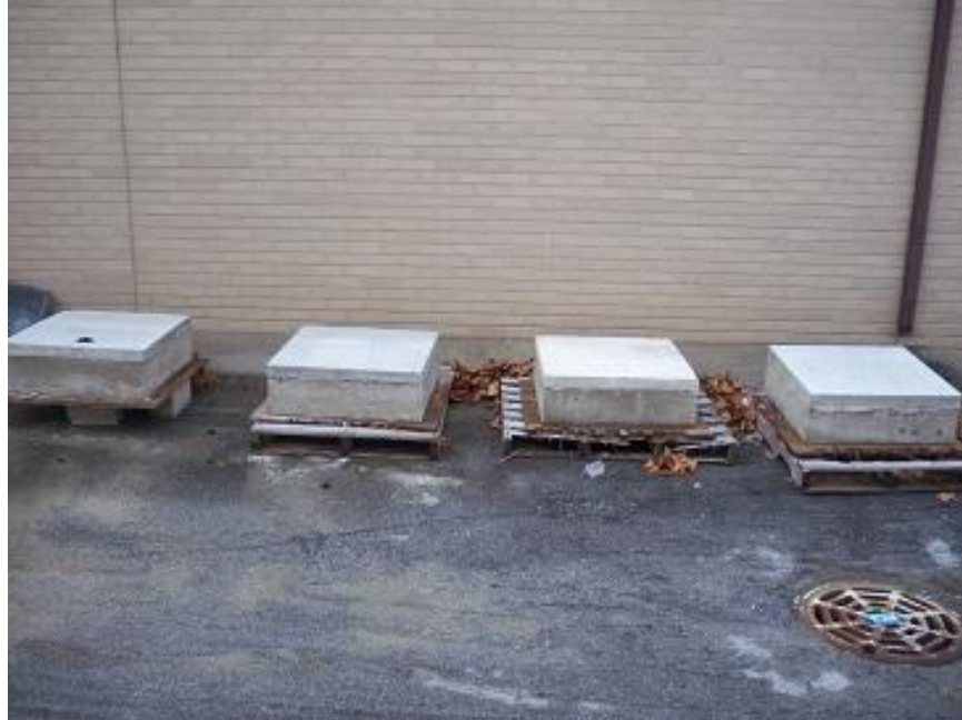
Figure 3.18. Four segments in an open environment (plain LMC, LMC-2SX+1GF, MSC-2SX+1GF, and FAC-2SX+1GF).
