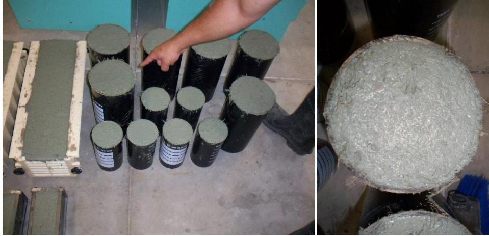
Figure 3.1. Portion of NXL fiber floated on the surface of the cylinders.
