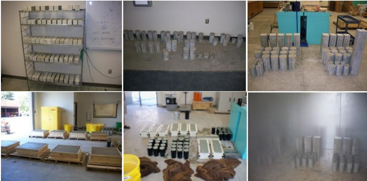
Figure 2.2. Preparation and curing of test specimens (not all steps shown).
