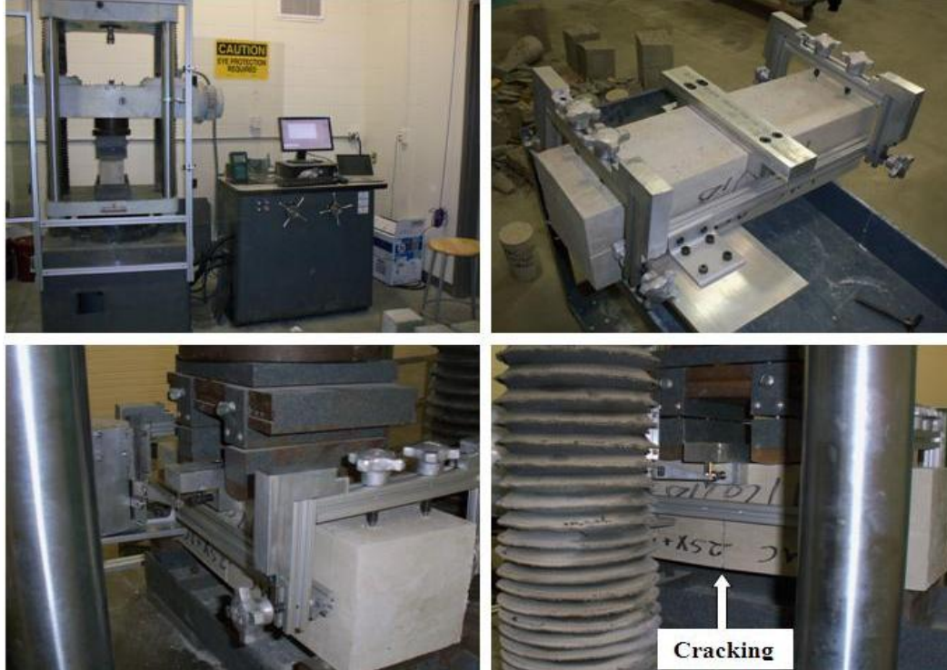
Figure 3.20. Testing machine, transducer arrangement, and cracking of a beam during ASTM C1609 toughness test.
