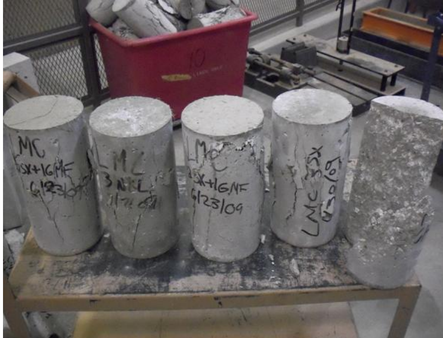
Figure 3.2. Failure modes of fibrous LMC (left four) and the plain LMC (right).
