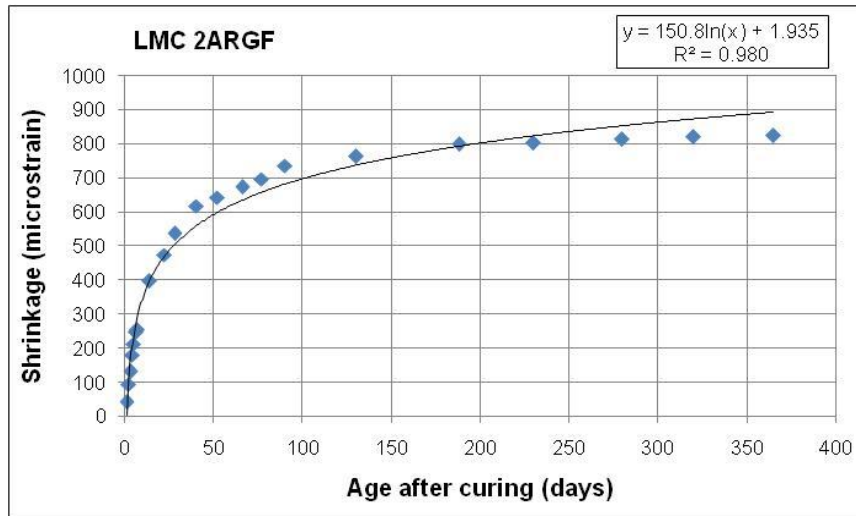
Figure 3.5. Shrinkage-time response of the LMC-2ARGF mixture.
