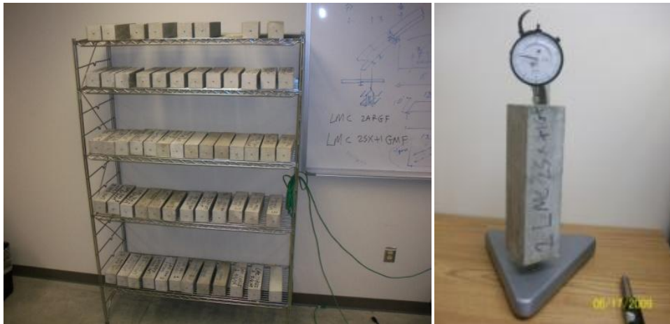
Figure 3.3. Shrinkage test prisms and mechanical dial indicator.
