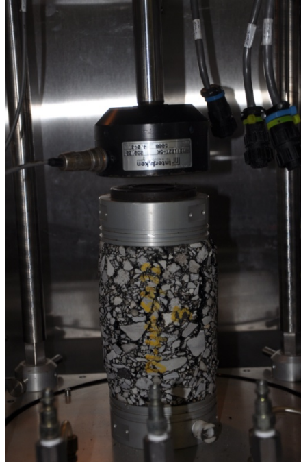
Figure 3.7. A specimen at the conclusion of a flow number test.
