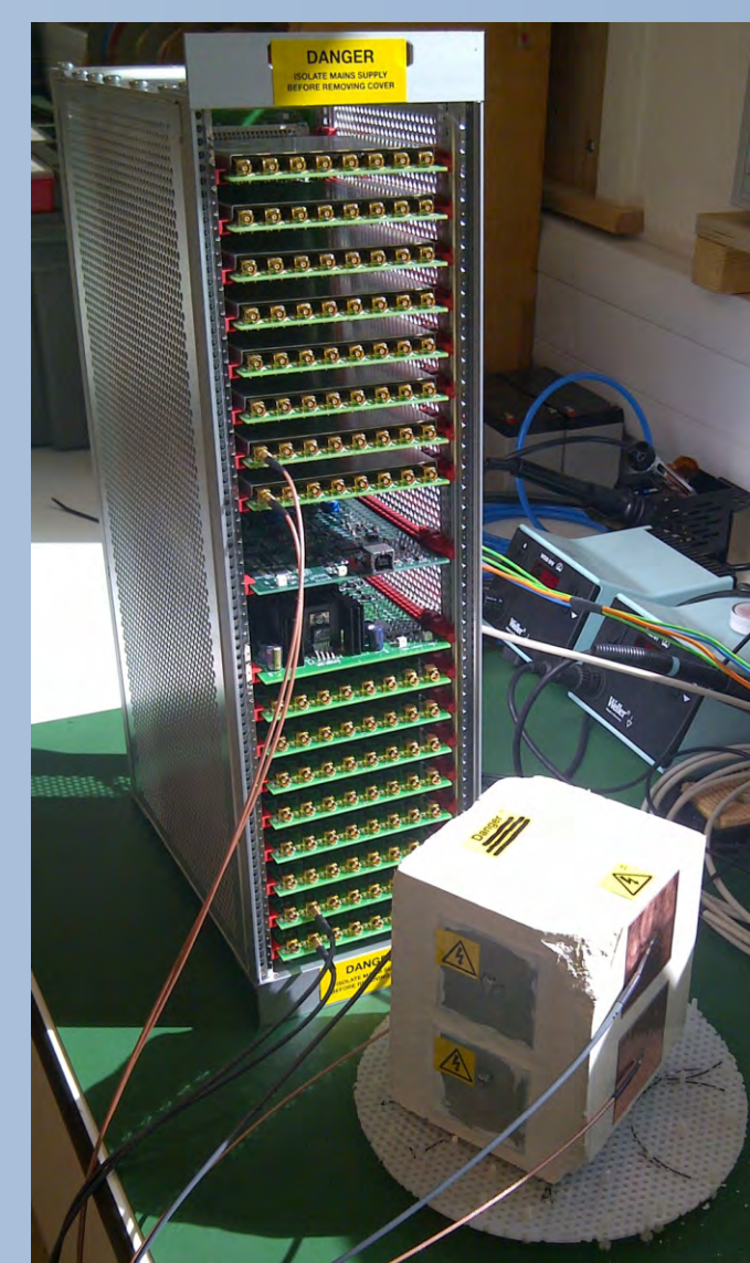
Figure 6: Prototype CRI instrumentation attached to sample of Newhaven Chalk, which has been instrumented with a four-plate capacitive sensor arrangement to determine resistivity.
