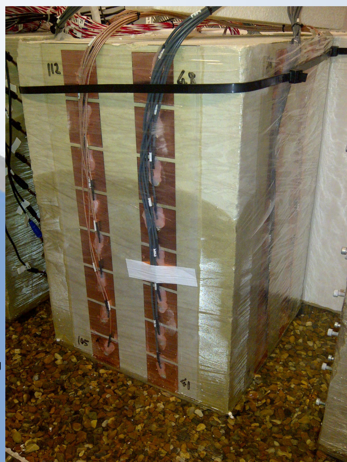
Figure 4: Rock sample instrumented with a capacitive sensor network allowing 4D capacitive resistivity imaging. A wetting front is clearly visible.
