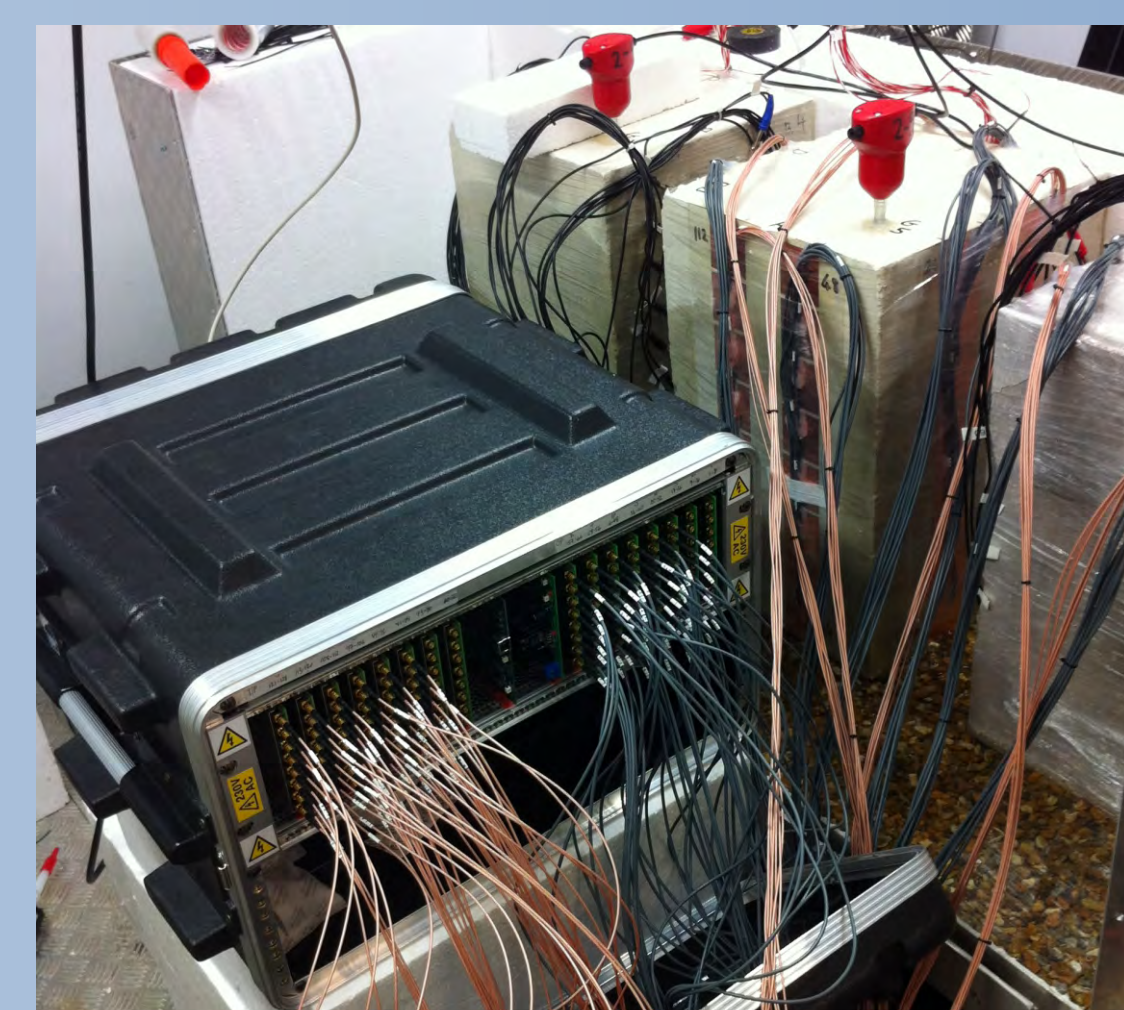
Figure 6: Prototype CRI instrumentation attached to sample of Newhaven Chalk, which has been instrumented with a four-plate capacitive sensor arrangement to determine resistivity.
