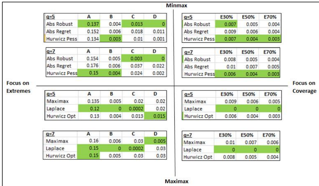
Figure 6: Average utility loss of different robustness measures and scenario sets for different numbers of uncertainties. The shaded cells indicate the lowest utility loss for a given scenario set. Numbers rounded to 3 d.p.
