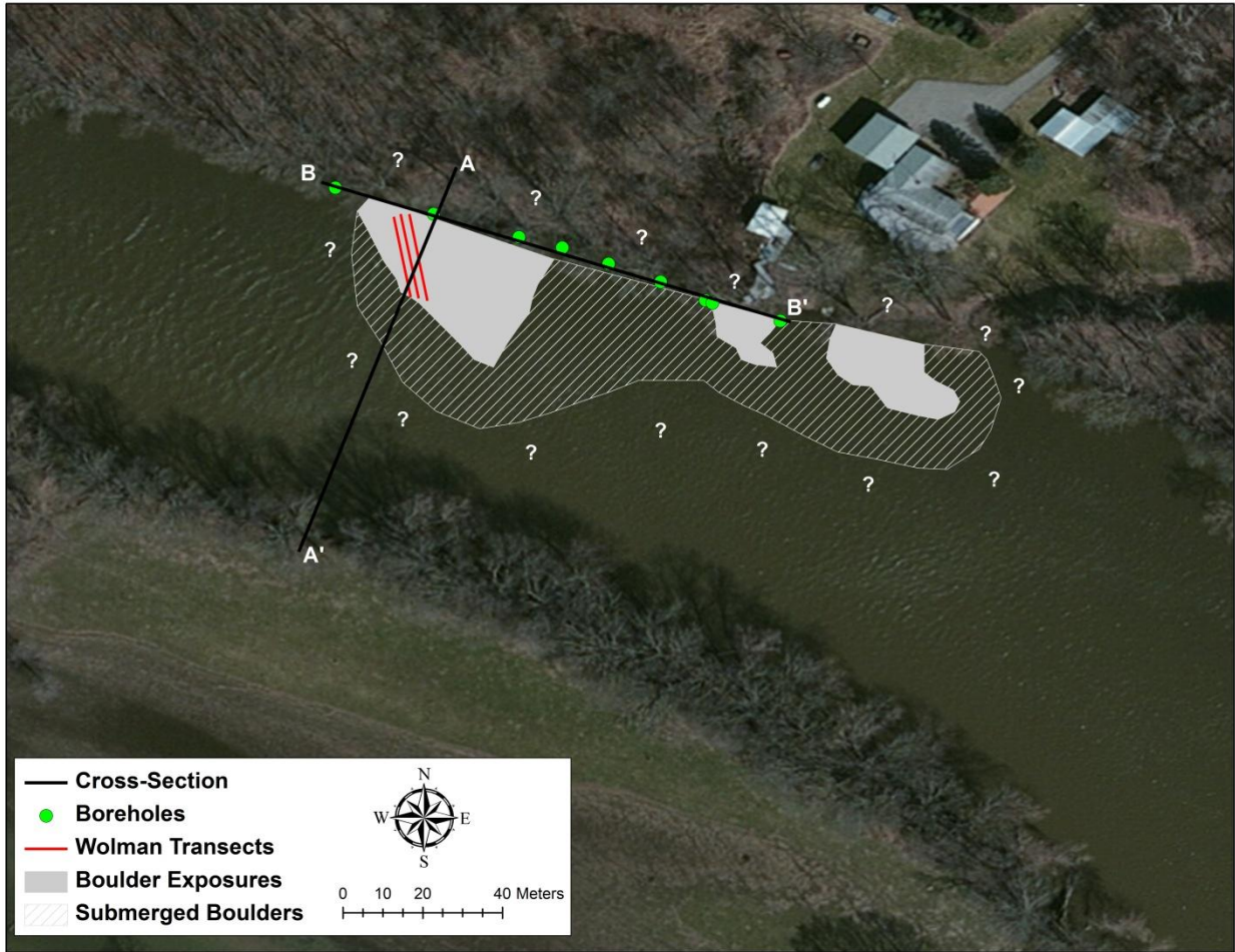
Fig. 9. Map showing the location and extent of the boulder-rich alluvium deposit and survey data used to characterize it. It is not known how far this deposit extends outside of the mapped area, as represented by question marks on the map
