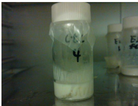
Figure 33. Syneresis in a cream vial from the CT50 group observed on day 3.
