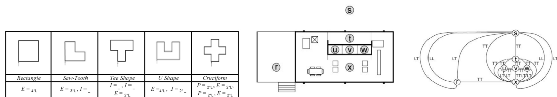
Figure 4. Q-code semantics and semantic graphs (Gero and Jupp, 2003, p.8, Jupp and Gero, 2003, p.4) Q-code semantics for primitive shapes (left), original drawing (centre) and semantic graph representation of Farnsworth House (right).
