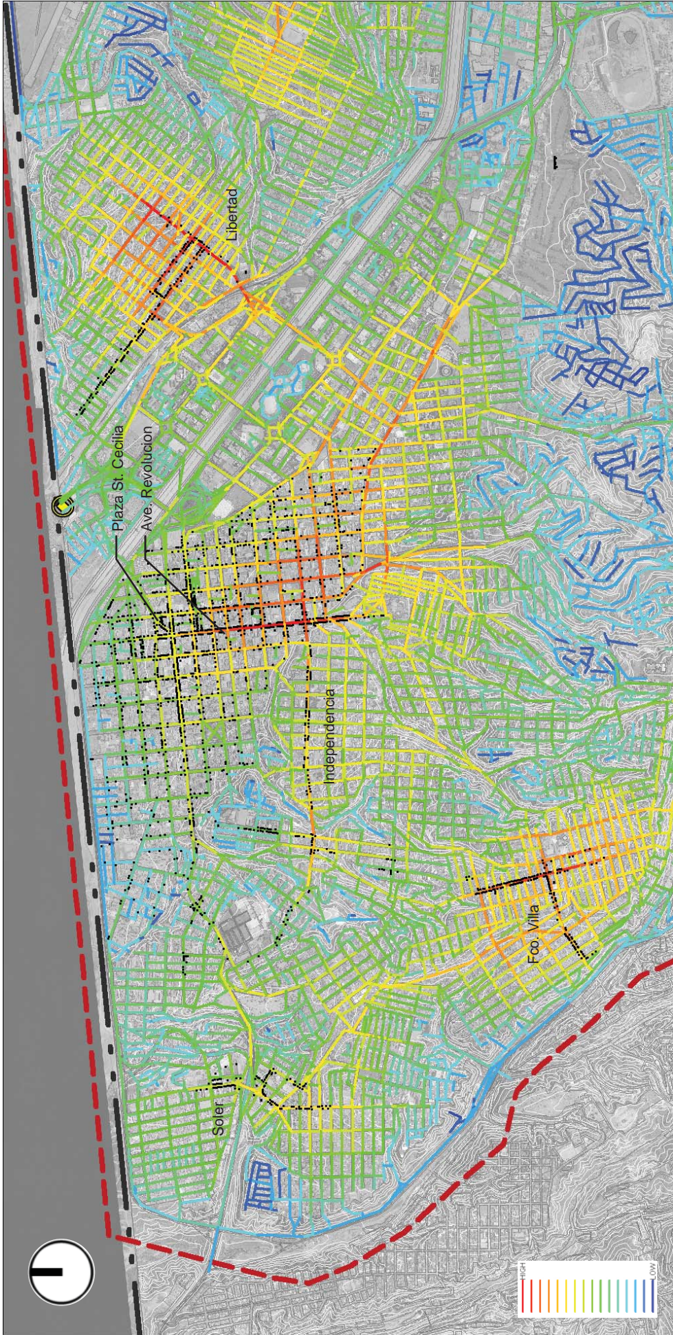
Figure 15. Study Area. Segment map showing Integration @ metric radius 1250. Source: IMPlan and Author. Map by: Author.
