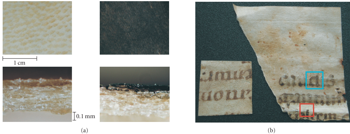
FIGURE 2: Samples used for examination: (a) preliminary samples and their cross-sectional views—on the right: sample covered with iron gall ink; on the left: a reference sample without ink; (b) samples of historical parchment with gall ink inscriptions.
