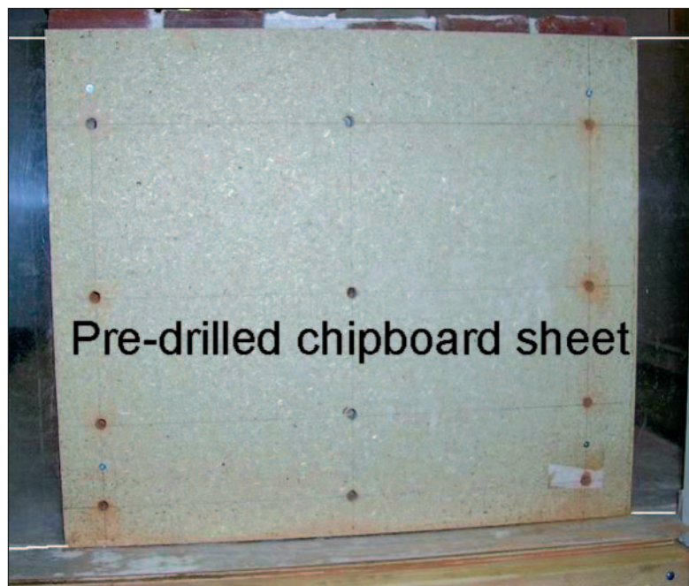
Figure 9 Template for drilling holes for sensors
