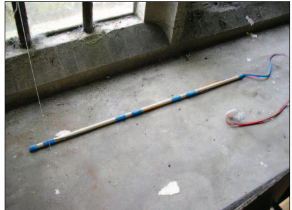
Figure 5 Replacement dowel with three measurement locations. Blue heat shrink sleeving is used to cover electrical connections.
