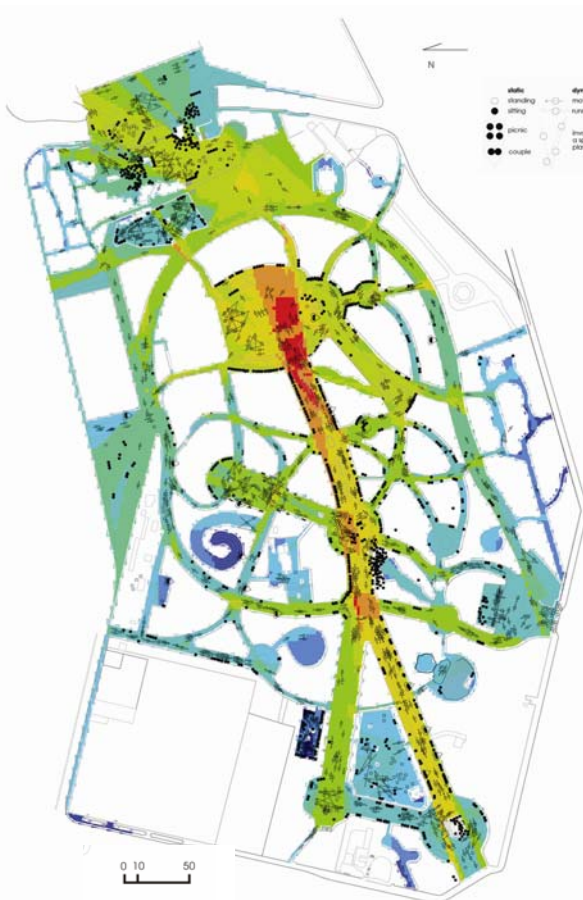
Figure 31: Visibility graph analysis of PA overlapped with combined snapshot data from five time periods
