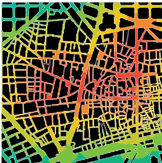
Fig. 4.5 Route C: Visual step depth metric shortest path colour range red=0 blue=1500
