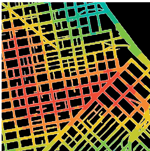
Fig. 7.5 Route D: Visual step depth metric shortest path colour range red=0 blue=1500
