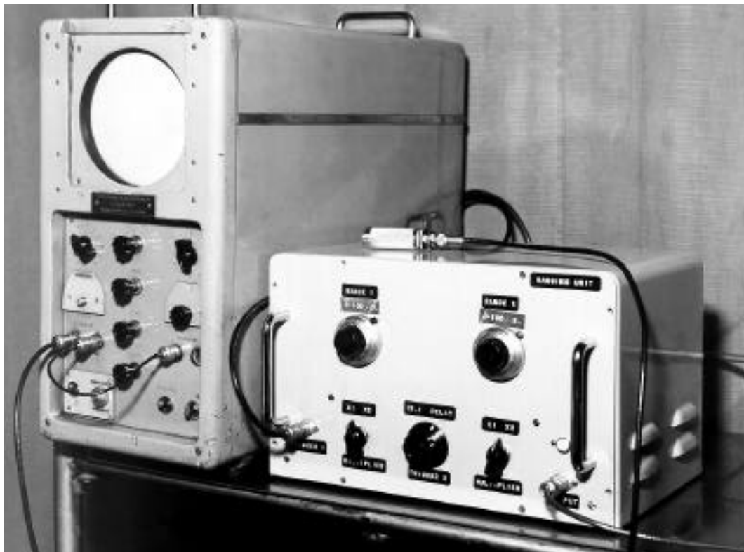
Figure 15. The apparatus in use for fetal cephalometry (head measurements) by ultrasound.
