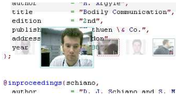
Figure 2: The user interface to the client application. Each contact of the user is represented by a video snapshot, rendered semi-transparently over the desktop. Offline contacts are represented by static images. On entering a video conversation the image becomes larger and opaque.
