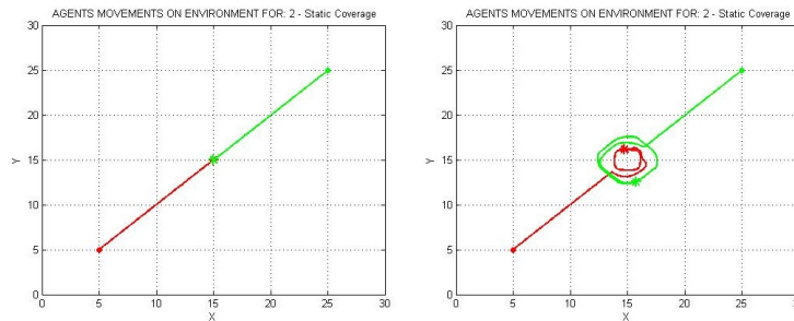
Fig. 4.9: Static Coverage with(right) and without(left) Collision Avoidance
