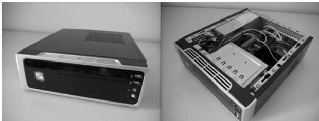
Fig. 2. Suitable HW platform containing x86 Intel Atom D410 1.66 GHz, RAM 1GB/677MHz and 16GB SSD
