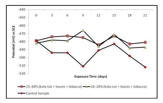
**Figure 9:** Variation of potential with exposure time for the mild steel specimen immersed in acid chloride, with varied percent concentrations of added kola nut, kola leaf and tobacco extracts. (KN, KL, TB = Kola nut, Kola leaf and tobacco extracts)
