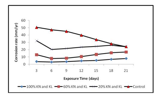
**Figure 2:** Variation of corrosion rate with exposure time for the mild steel specimen immersed in acid chloride, with varied percent concentrations of added kola nut and kola leaf extracts. (KN, KL = kola nut and kola leaf extracts respectively)
