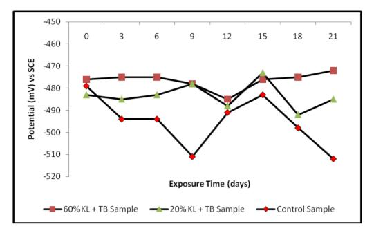
**Figure 8:** Variation of potential with exposure time for the mild steel specimen immersed in acid chloride, with varied percent concentrations of added kola leaf and tobacco extracts. (KL, TB = Kola leaf and tobacco extracts)
