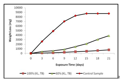
Figure 3: Variation of weight loss with exposure time for the mild steel specimen immersed in acid chloride, with varied % concentrations of added kola leaf tobacco extracts.
