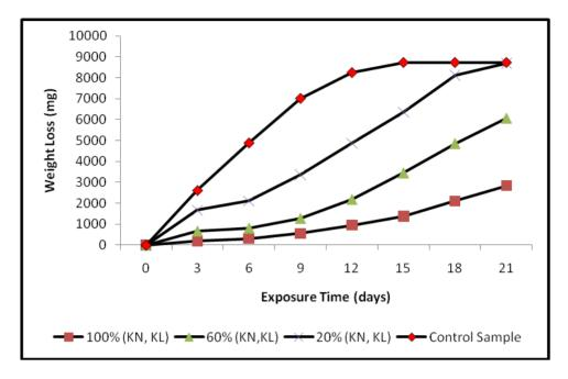
**Figure 1:** Variation of weight loss with exposure time for the mild steel specimen immersed in acid chloride, with varied percent concentrations of added kola nut and kola leaf extracts. (KN, KL = kola nut and kola leaf extracts respectively)
