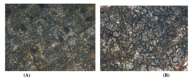
**Figure 10:** Mild steel test specimen: (a) and (b) after 21- day immersion in 60% kola leaf; and in 100% kola nut and tobacco leaf extracts concentrations respectively.
