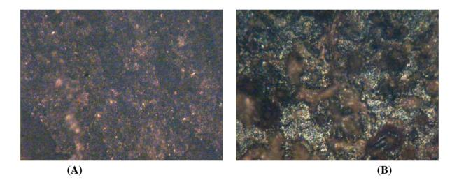
Figure 11: Mild steel test specimens: (a) after 21 day immersion in 60% concentrations of added kola leaf and tobacco; and (b) 21 days in 60% concentrations of added kola nut, kola leaf and tobacco extracts respectively.
