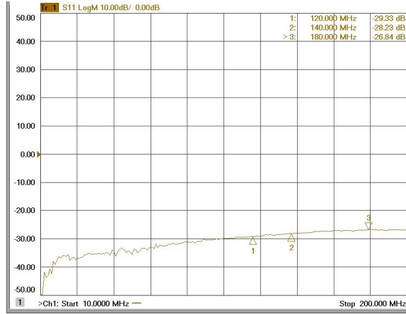
Figure 6.14: Return Loss of the RF port of Bias-Tee
