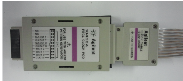
Figure 4.16: Clock cable connected to a Clock pod
