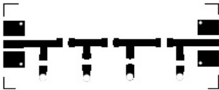
Figure 6.3: Low Pass Filter PCB Layout
