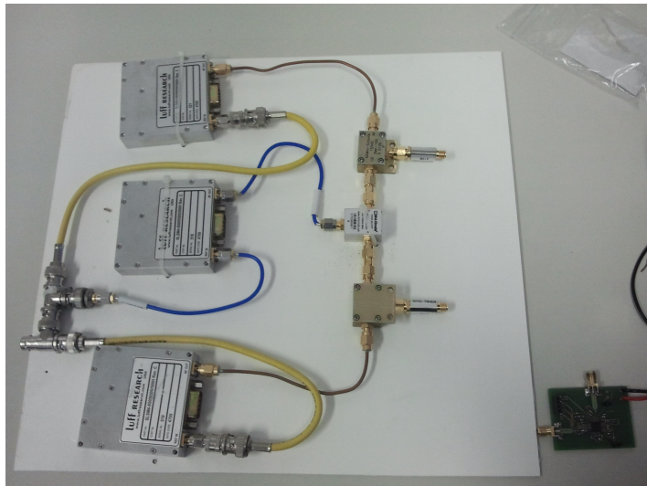
Figure 3.14: CW Generator solutions
