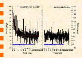
The evolution of the state of the plasma can be monitored real-time by displaying changes in phase and amplitude.
