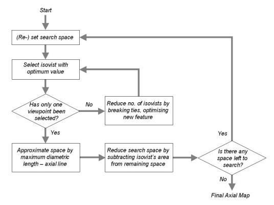
Figure 4: Generic Algorithm for Sorting Isovists and Generating Axial Maps
