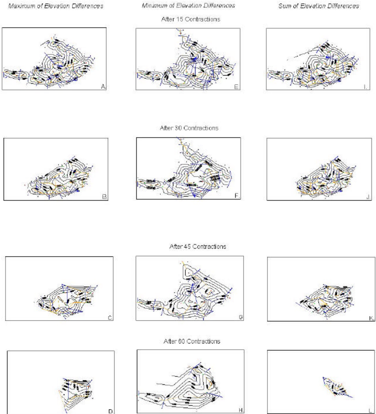
Fig. 7 Surface Networks and respective contour maps (200m interval) of Latschur surface network after each 15 contractions based on maximum of elevation differences criterion (A-D), minimum of elevation differences criterion (E-H) and sum of elevation differences criterion (I-L).
