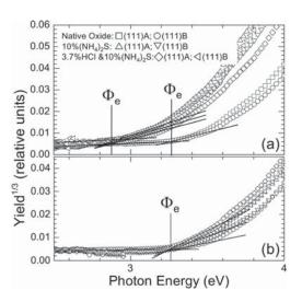
FIG. 3. Cube root of the IPE yield, measured with the average strength of electric field in the oxide of 1 MV/cm, at the interfaces of p-doped (a) and n-doped (b) GaAs(111) samples with an Al<sub>2</sub>O<sub>3</sub> layer for different surface orientations and pre-ALD treatments. The vertical lines mark the inferred thresholds,  $\Phi_e$ , of electron IPE from GaAs into Al<sub>2</sub>O<sub>3</sub>.
