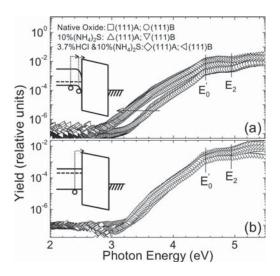
FIG. 2. Semi-logarithmic spectral plots of the IPE yield as a function of photon energy measured, under +2.0 V bias applied to the Au electrode, on p-type (a) and n-type (b) GaAs(111)/Al<sub>2</sub>O<sub>3</sub>/Au samples for different surface orientations and pre-ALD treatments. The vertical lines indicate energies of optical singularities in the GaAs crystal. Insets show a schematic of the observed electron transitions.
