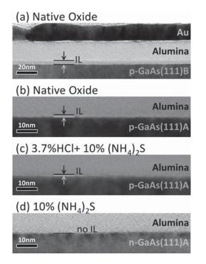
FIG. 1. Cross-sectional TEM images of the interfaces prepared by ALD of  $Al_2O_3$  onto p-type GaAs(111)A and GaAs(111)B surfaces covered with native oxide [panels (a) and (b), respectively] and of the p-GaAs(111)A/ $Al_2O_3$  interface prepared by etching the native oxide in HCl followed by sulphur passivation (c). For comparison is shown the image of an IL-free interface obtained on a sulphur passivated n-GaAs(111)A surface (d).
