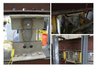
Throughout the project, the test specimen (left) was used for full-scale experimental tests as well as the heaters (top right), together forming the full test setup (bottom right).
