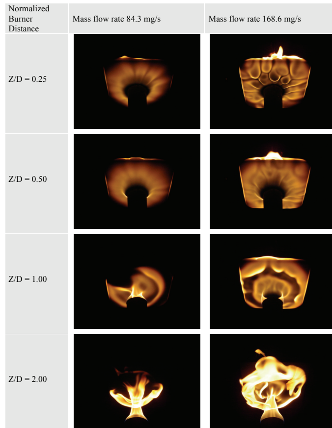
Figure 3. Qualitative images of visible radiation emitted by the propane ( C_3H_8 ) impinging flame for a range of plate positions and fuel mass flow rates.
