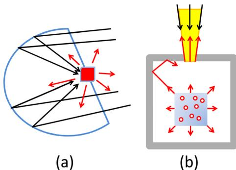
Fig. 7. (a) Angle broadening of incident photons using a solar concentrator; (b) a scheme limiting the emission angle of the PV system.
