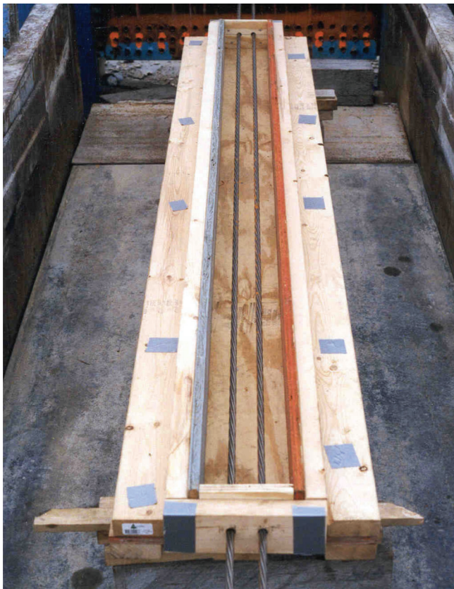
Figure 3.30 Formwork and prestressing strands for transfer length specimen.
