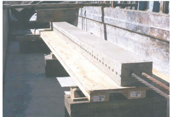
Figure 3.31 Whittemore points mounted on a transfer length specimen.
