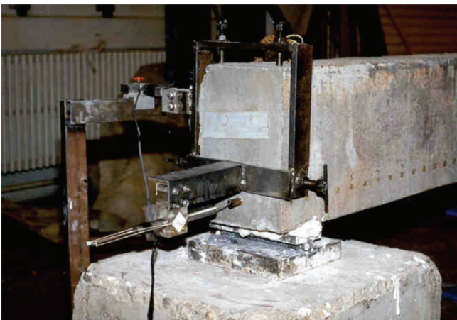
Figure 3.35 Strand slip measuring device for single-strand development length beams.
