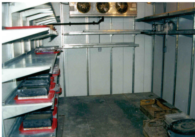
Figure 3.9 A view of the setup in the freeze-thaw room used for testing deicing salt scaling specimens.
