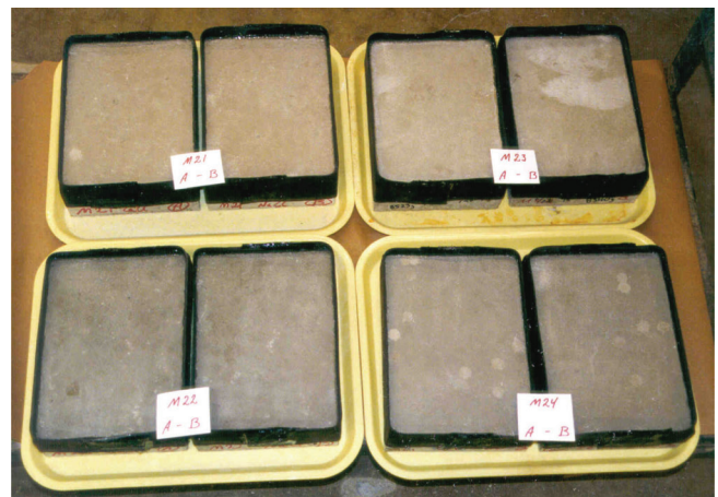
Figure 3.10 Four sets of deicing salt scaling specimens prior to freeze-thaw testing.
