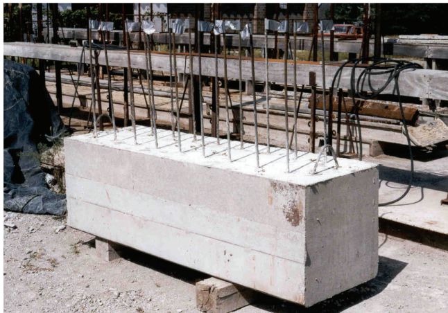
Figure 3.28 Pullout specimen before testing of strands.
