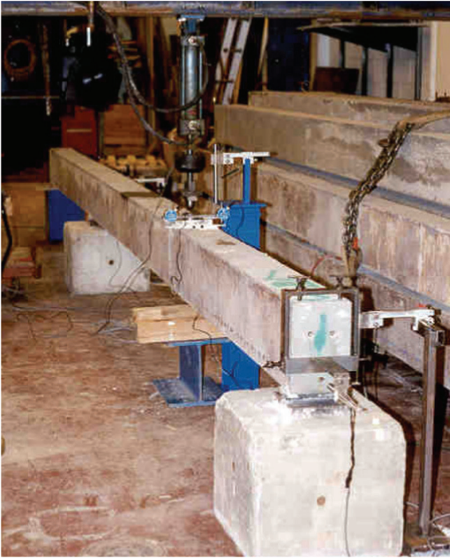
Figure 3.34 Test setup for a single strand development length beam.
