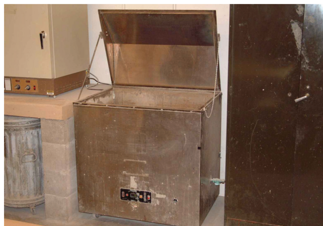
Figure 3.11 Water heater used for accelerated curing of deck field trial specimens requiring curing in lime water at 38^{\circ}\text{C} ( 100^{\circ}\text{F} ).
