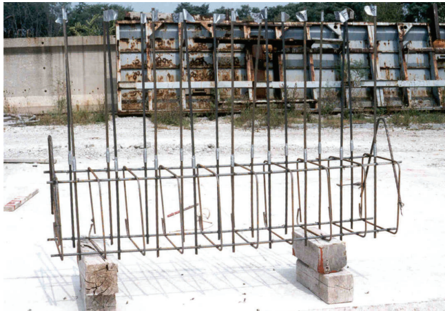
Figure 3.27 Reinforcement cage and strand specimens used in the pullout specimen.
