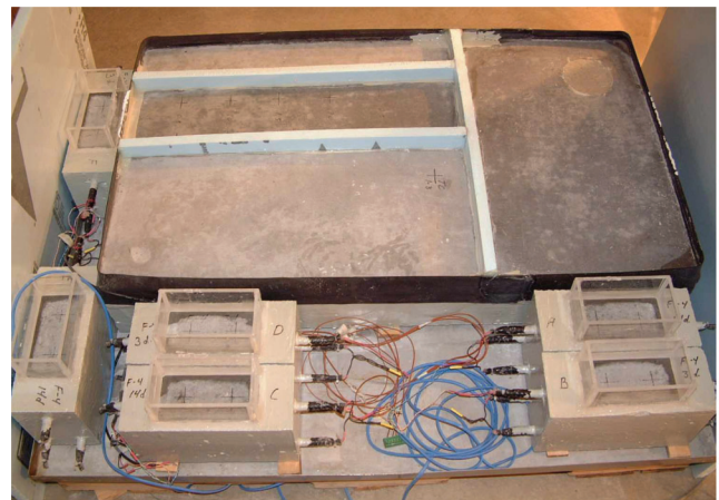
Figure 4.58 Corrosion specimens from mixture F-4. Partitions on ponding slab were used to prevent salt solution from entering cracks above small sheets of Plexiglas used to support ladder macrocells.
