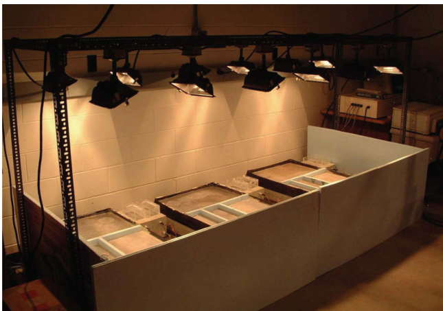
Figure 3.16 Experimental setup of halogen heat lamps and corrosion specimens during the drying portion of the weekly exposure cycle.
