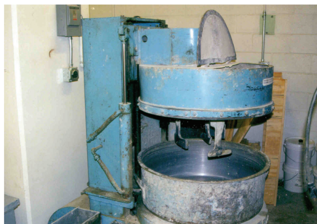
Figure 3.1 Counter current pan concrete mixer used to mix all concrete made in the laboratory.
