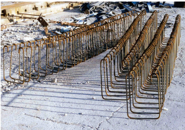
Figure 3.47 Stirrup assemblies used below the longitudinal strands in the multiple-strand development length specimens.
