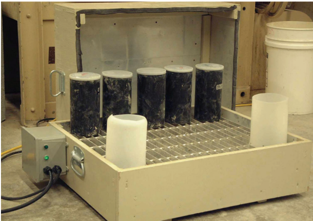
Figure 3.23 Temperature matched curing enclosure with five 102×203mm (4×8in.) cylinder molds and two ducts for facilitating movement of air from two of the fans to the top of the enclosure.
