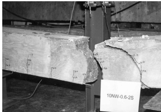
Figure F.12 Single-strand development length specimen 2S after failure.
