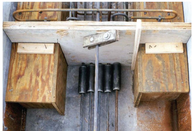
Figure 3.40 Splicing of Insteel and Florida Wire & Cable strands.
