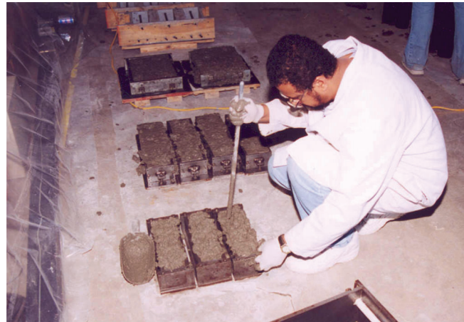
Figure 3.22 Preparation of three shrinkage specimens by rodding.
