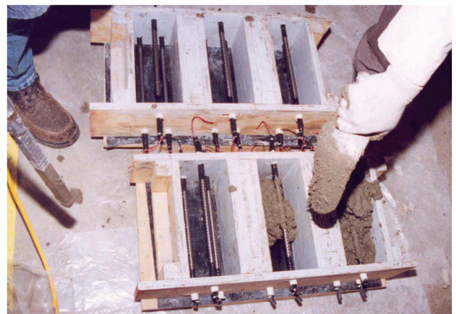
Figure 3.14 Preparation of six beams used for corrosion testing.
