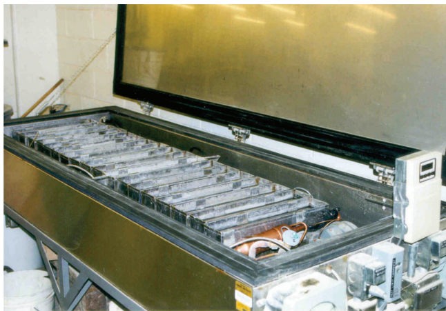
Figure 3.5 Freeze-thaw machine used for rapid freezing and thawing of specimens under water.
