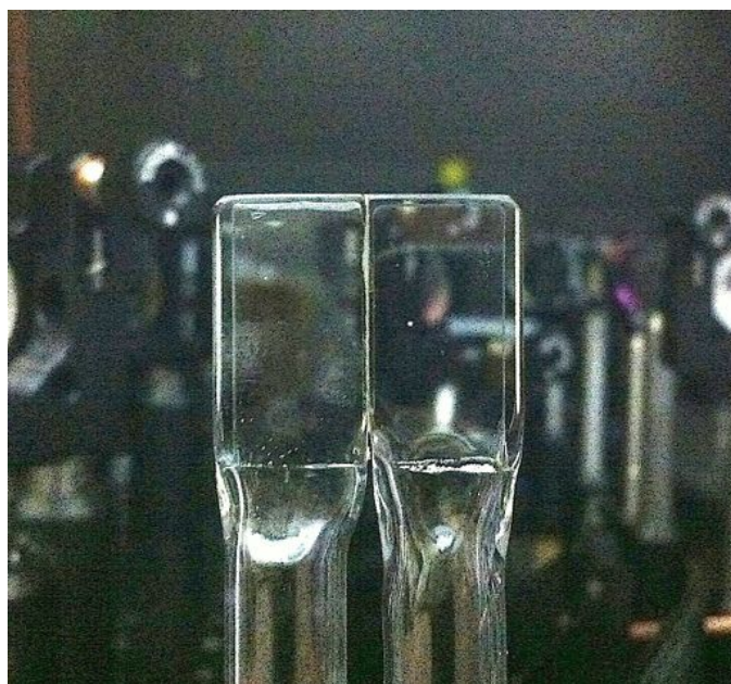
Figure 9.1.: Multi-region 2 mm vapour cell developed in collaboration with the Chemistry Department at Durham University. The separation between the chambers is approximately 800 \mu\text{m} .
