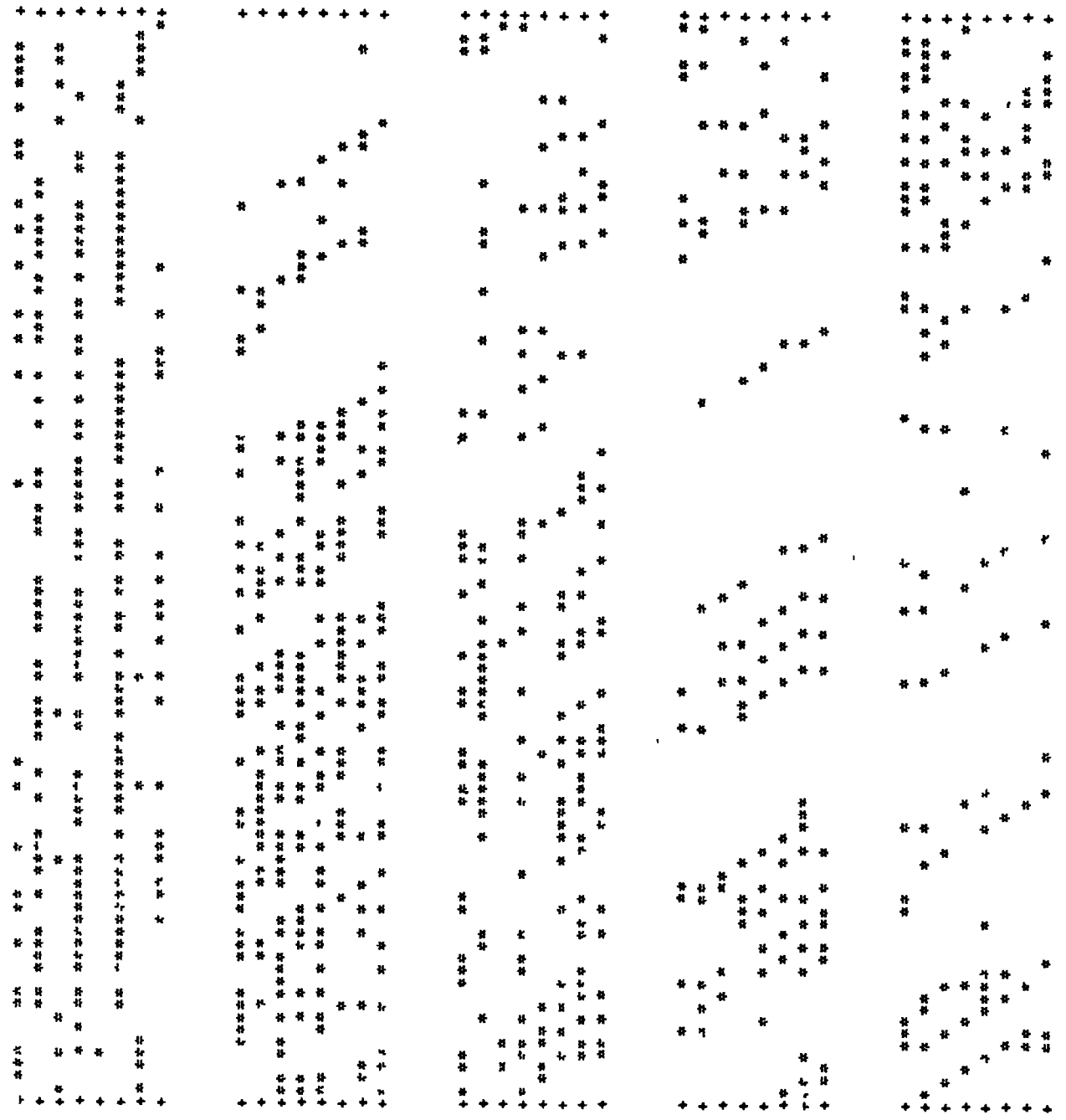
Figure 3.15 A large angle ( \sim 30^\circ ) shower causing a high density of discharged tubes in all the measuring trays.
