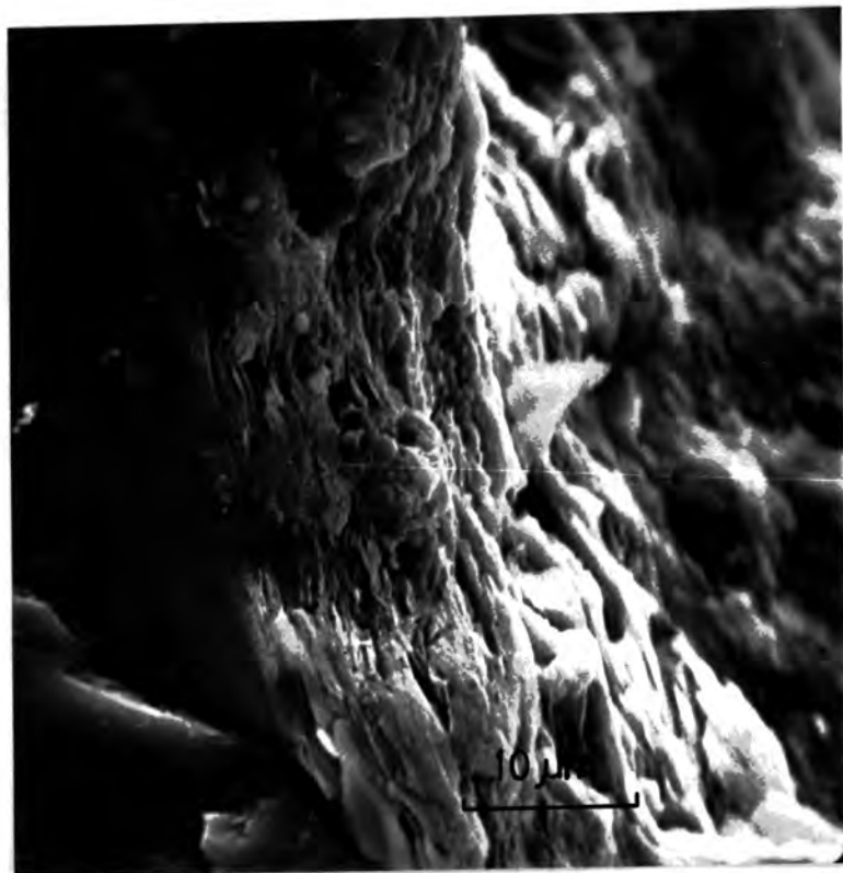
C. Detail of mica cleavage planes showing perhaps traces of matrix material still adhering.
