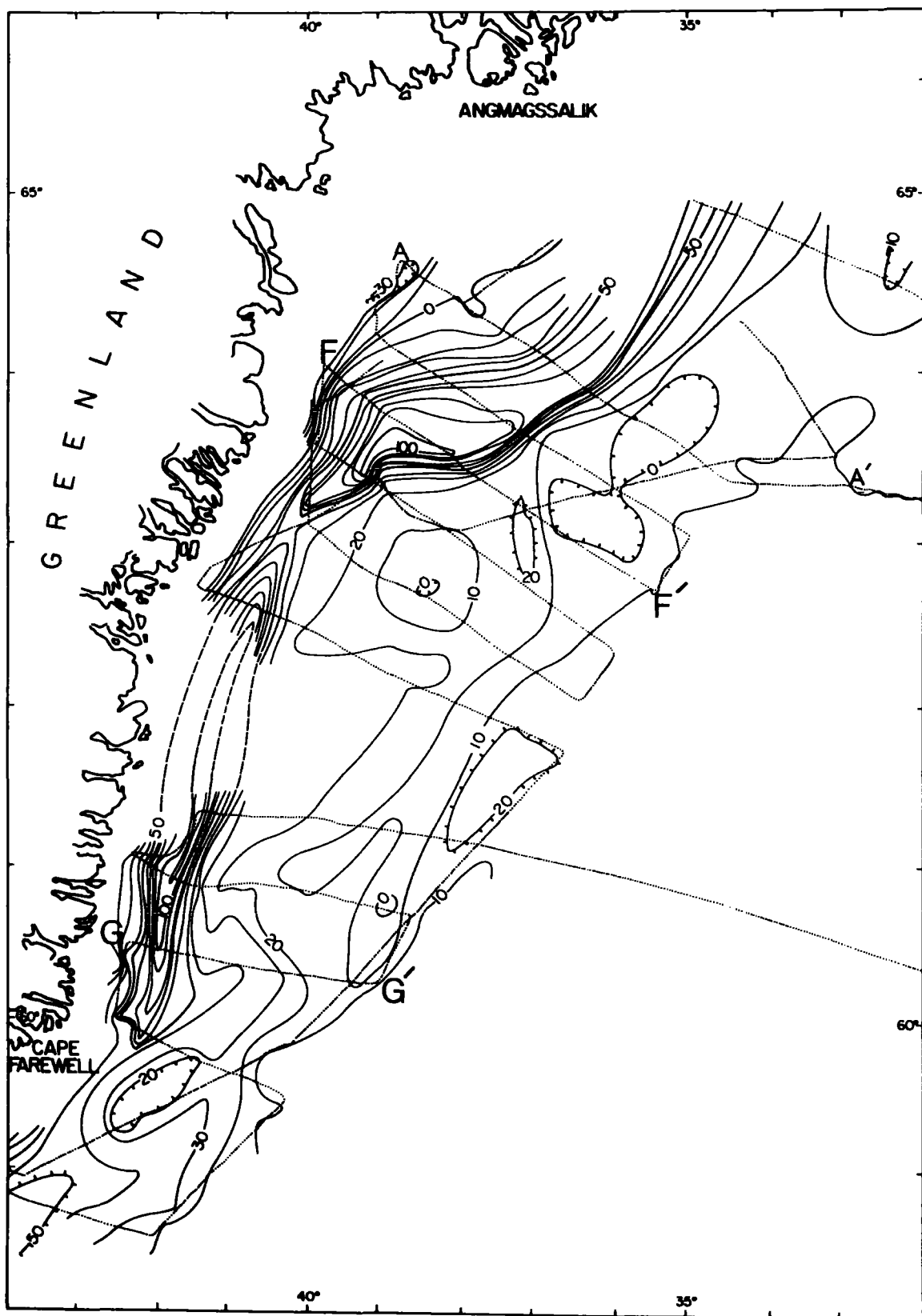
Fig. 6.1 Free air gravity anomaly map of the south-east Greenland margin. Contour interval 10 mgal, ship's track as dotted lines.
