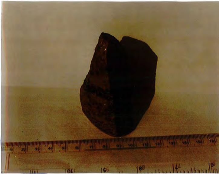
Plate 2.11 Chromite rich band in dunite. Note the irregular, wavy boundaries of the band and the sharp alternation to bare dunite.
