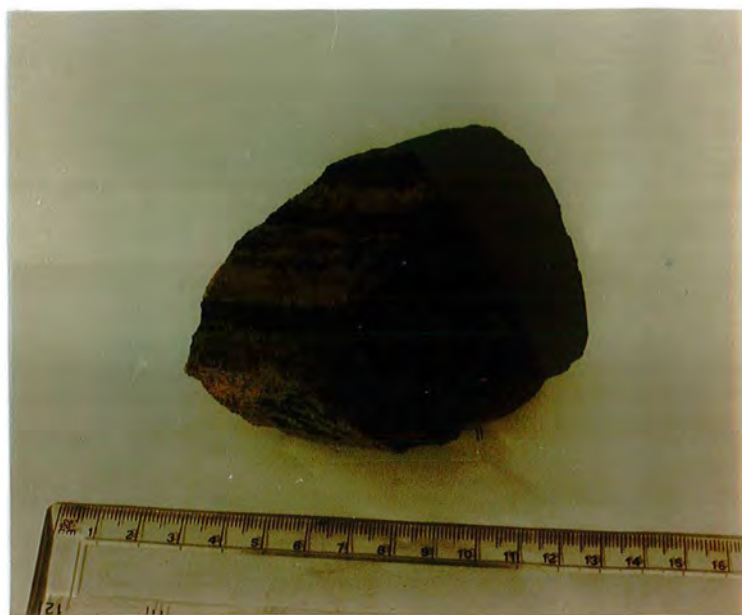
Plate 2.8 Massive chromitite bands commence from a chromite-rich rod. Chromitiferous dunite forms between the massive chromite bands and at the bottom of the sample. Note the dunite formation between the chromititic bands.
