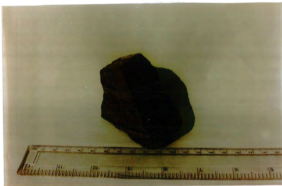
Plate 2.5 Disseminated type ore. Rich in chromite bands alternate with bare dunite. This sequential repetition suggests magmatic origin.
