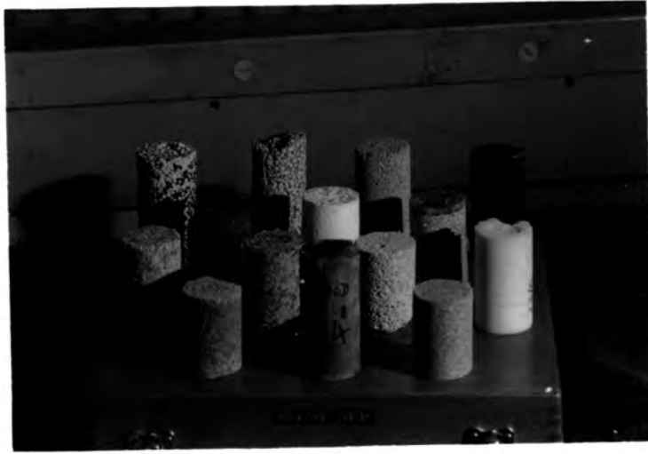
2" cylinders compacted in the laboratory. Black one was a bituminous specimen
