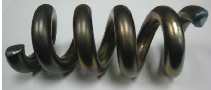
Figure 2.14: The SMA helical spring used in the experimental study.
