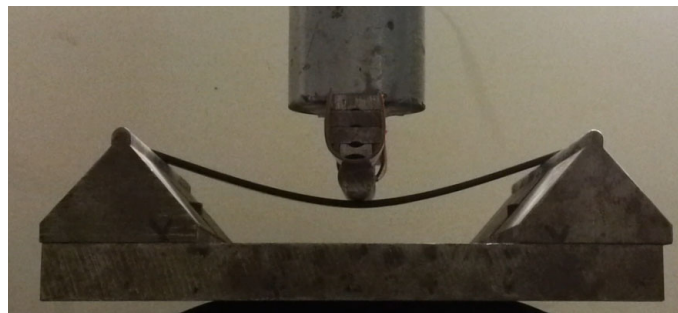
Figure 2.60: The experimental setup for the three-point bending test of an SMA beam.
