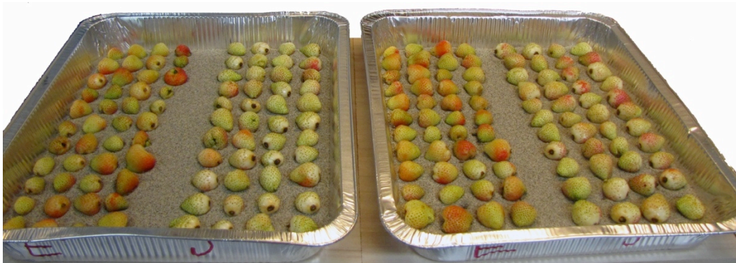
Figure 5.4. Moist chamber set up to carry out pathogenicity assays on strawberry fruit. Sets of two trays were considered as a single replication.
