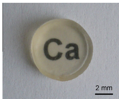
Fig. 3. Hybrid of 40 wt.% 120 kDa \gamma\text{CaPGA} , where every tenth repeating unit of \gamma\text{PGA} was functionalized with GPTMS.
