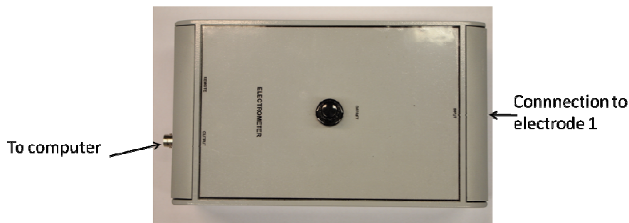
Figure 2.5 A home-built high sensitivity current follower.
