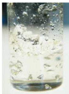
Figure 5.2: Gel formed on polymerisation of EGDMA/GMA (90/10 mol%) in 1,2-dichloroethane, swollen in additional 1,2-dichloroethane
