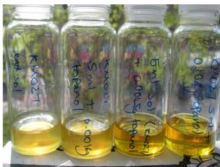
Figure 2.7: EGDMA homopolymers with varying amounts of antioxidant. From left to right- no BHT, 0.03% BHT, 0.16% BHT, 3.5% BHT in 5 ml (approx 2.5 mL polymer) of polymer solution.
