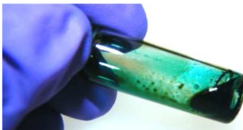
Figure 3.5: Colour change of CoBF from orange/brown powder to green/blue solution on the addition of pure colourless DMPP
