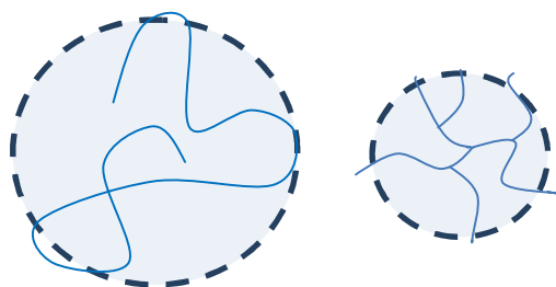
Figure 2.1: Illustration of the difference in hydrodynamic volume of a linear and branched polymer in solution
