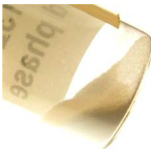
Figure 5.4: Polymer from the CCTP of EGDMA/GMA (50/50 mol%) in acetonitrile, 50% solids, after precipitation in hexane
