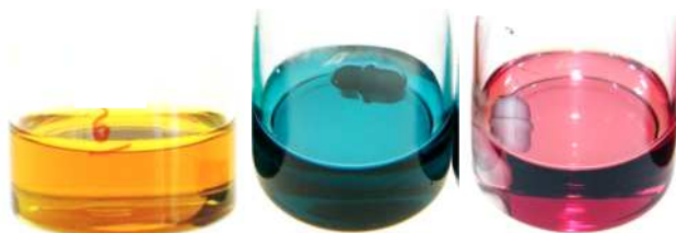
Figure 5.19: Colour change of poly-EGDMA homopolymer (yellow) on addition of functional primary amines (green/blue) and colour change on heating solution at 60 °C for 24 hours (red)
